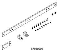
Mount horizontally on rack, providing a convenient place to connect equipment grounds. Made of electrolytic tough-pitch 110 copper alloy. Kits include ground bar with mounting hardware, eight #6-32 x 14 machine screws, and eight #6 ring terminals.
