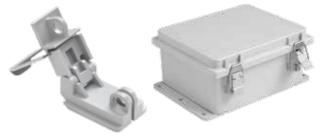
Stainless Steel Latches can be retrofitted on all POLYPRO models with no modification or drilling required. Hinge/latch constructed of corrosion-resistant polyester with a Type 316L stainless steel bail.
