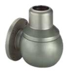
Wall Joint with vertical socket for mounting to vertical surfaces. Cover to facilitate wiring. Turns through 340 degrees with rotation limiter. Preset torque. Maintenancefree bearings. Type 304 polished stainless steel finish. Includes gaskets. Wall-mounting fasteners not provided.
