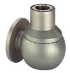
Swivel Wall Coupling for direct mounting of enclosure to vertical machine surfaces. Turns through 340 degrees with rotation limiter. Cover to facilitate wiring. Preset torque. Maintenance-free bearings. Type 304 polished stainless steel finish. Includes gaskets and enclosure mounting hardware. Wallmounting fasteners not provided.
