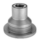
Swivel Base External Bracket Coupling for mounting enclosures directly to a machine or the floor. Turns through 340 degrees with rotation limiter. Preset torque. Maintenance-free bearings. Type 304 polished stainless steel finish. Includes gaskets and enclosure mounting hardware. Base-mounting fasteners not provided.
