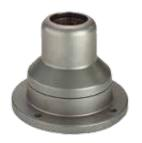
Swivel Base for mounting to machine or floor. Turns through 340 degrees with rotation limiter. Preset torque. Maintenance-free bearings. Type 304 polished stainless steel finish. Includes gaskets. Basemounting fasteners not provided.
