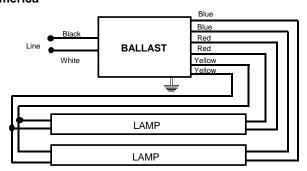
Ballast must be grounded in accordance with national and local electrical codes.
