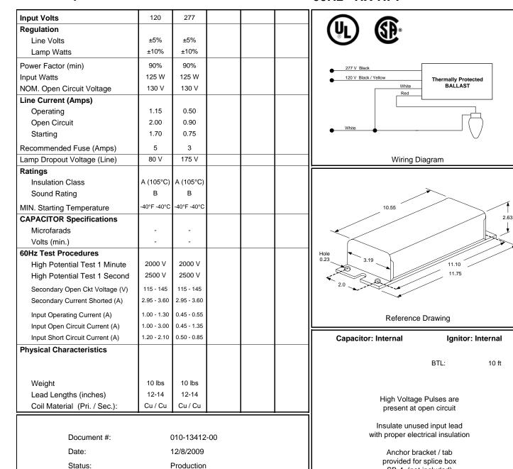
Data is based upon tests performed by Universal Lighting Technologies in a controlled environment and is representative of relative performance.
