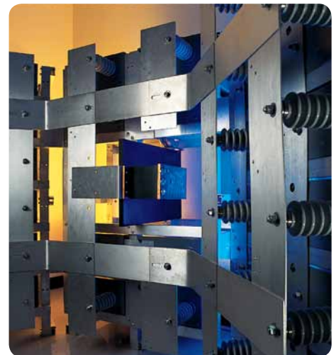
▲ Schneider Electric lightning generators test Surgelologic SPDs in real-world systems and situations.
