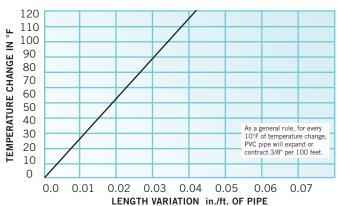
PVC Pipe Length Variation due to Temperature Change (°C) Coefficient =  $.054 \times 10^{-5} \text{ mm/m/°C}$
