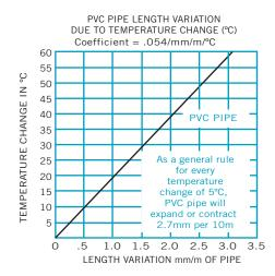
°C Total Expansion (mm) = length of run (m) x temperature change (°C) x 0.054
