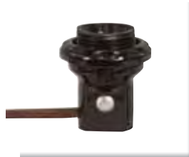
80-1473 1 1/4" with Shoulder and Phenolic Ring 24" 18/2 SPT-1 Brown Leads 105°C 75W-125V
