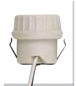
90-1107 Snap In Socket 8" AWM B/W Leads 105°C 660W-250V
