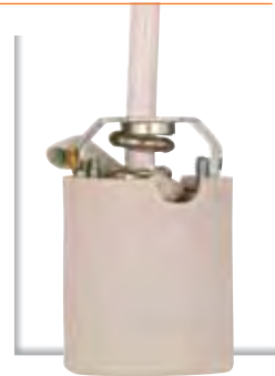
90-1563 White 90-1564 Black Porcelain Socket w/1/8 IP U-Bracket Hickey w/Strain Relief & Fiber Sleeving 8Ft. 18/3 SVT 105°C 660W-250V
