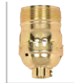
90-1412 Short Keyless 1/8 IP Cap w/Set Screw 660W-250V
