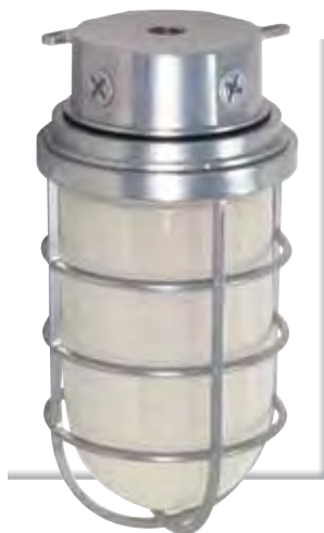
Large Metallic Silver 76-626 (1) 200W A Type max. Dimensions: Height 11", Diameter 5 1/2"
