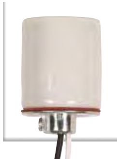
80-1313 Porcelain Socket w/1/8 IP Cap 9" AWM B/W Leads 150°C Pulled Thru Cap - 660W-250V
