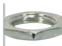
Steel Locknut – 1/4 IP 11/16" hex., 1/8" thick 90-1038 Unfinished 90-591 Brass Plated 90-171 Zinc Plated
