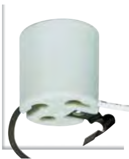
80-2652 Snap-In Socket Bracket Extends 3/8" from End of Socket 12" AWM B/W Leads 150°C 660W-250V
