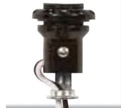
90-1557 1 3/4" with Shoulder and Phenolic Ring 8" AWM B/W Leads 105°C Pulled Thru 1/8 IP Inside Extrusion 75W-125V
