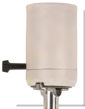
90-428 Three Way Turn Knob Mogul Base Socket Screw Terminals 1/4 IP Hickey 750W-250V
