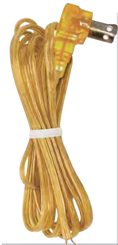
Flat Plug Cord Set 18/2 SPT-2 105°C Molded Plug Tinned Tips 3/4" Strip with 2" Slit 36" Hank
