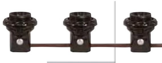
80-1474 1 1/4" with Shoulder and Phenolic Ring 6" Centers 18" Tail 18/2 SPT-1 105°C Brown 75W-125V
