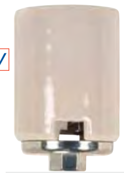
80-1378 Keyless Mogul Base Socket with Wireway Screw Terminals 1/4 IP Cap 1500W-600V 4KV Pulse Rated
