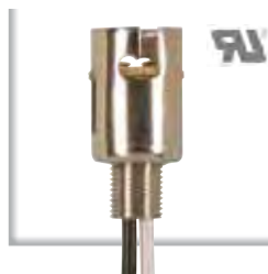
90-1558 1/8 IP Nipple 8" AWM B/W Leads 105°C Pulled Thru 150W-125V
