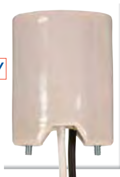
80-1377 Keyless Mogul Base Socket w/2 Mounting Screws 16"-SF-2 B/W Leads 200°C with Wireway 1500W-600V 5KV Pulse Rated
