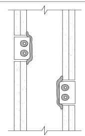
Putty pad reduces sound transmission by blocking path of sound travel.
