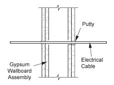
UL System No. W-L-3024 F Rating – 1 & 2 Hr • T Rating – 0,1/2, 1 & 2 Hr Electrical, Telephone or Data Cables Annulus: 0" to 1/4" Putty Depth: 5/8" of Putty on both sides.
