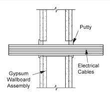
UL System No. W-L-3135 F Rating – 1 & 2 Hr • T Rating – 0 Hr Electrical, Telephone or Data Cables Annulus: 1/4" to 3/4" Putty Depth: 5/8" of Putty on both sides.
