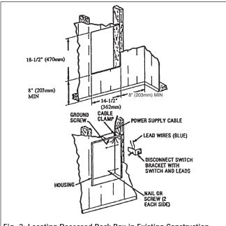
Fig. 2: Locating Recessed Back Box in Existing Construction
