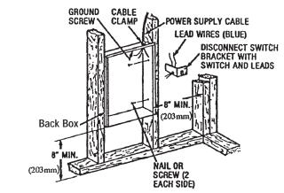
Fig. 1: Locating Recessed Back Box in New Construction
