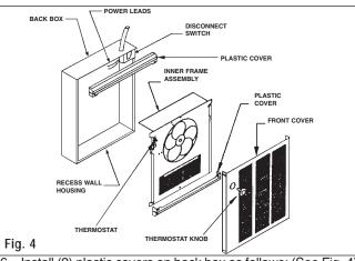
6. Install (2) plastic covers on back box as follows: (See Fig. 4) **NOTE:** Both top and bottom plastic covers are identical.
