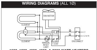
**1500, 1800, 4800, 4000, & 3000 WATT HEATERS**120V, 208V, 240V, OR 277V (Full wattage heaters can be converted to half wattage by removing the red jumper wire connecting the top and bottom element terminals.)
