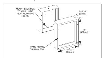
Fig. 3: Optional Surface Mounting Frame Installation
