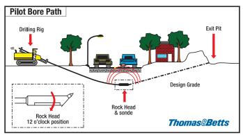
Bore-Gard® can be used under highways without disrupting traffic.
