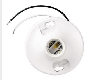
Medium base, phenolic, one-piece keyless, 4 terminals with tri-drive scews, fits 3 1/4 and 4" boxes, with cage necks, 6" Leads. White.
