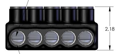
WIRE ENTRY POINT WIRE RANGE: 250 - #6AWG PRE-FILLED W/ OXIDE INHIBITOR-
