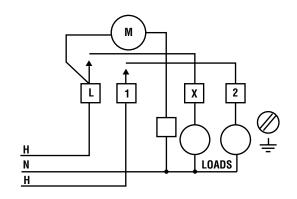
Disconnect power at main panel prior to installing or servicing this time switch or the equipment connected to it. Connect in accordance with national and local electrical codes.
