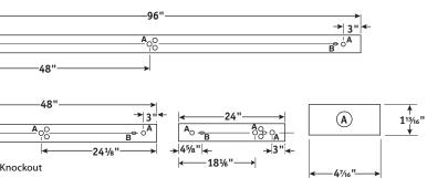
te 1: All Non-Shielded (strip) fixtures- Deduct ۱٬۱۵" from overall dimension for continuous row mounting. mensions shown include end panel.
