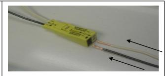
DIAGRAM 4 – Insert solid conductor supply wires into luminaire disconnect plug.
