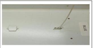
DIAGRAM 2 – Thread geartray tether into geartray.
