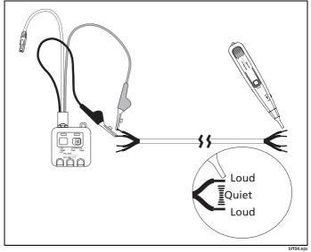
Figure 4. Tracing Pairs
