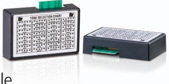
The UTM is a microcontroller-based tone generator capable of producing 32 different tones. The UTM is the key component of a SelecTone® System or a single SelecTone device. Tone selection is made by setting five DIP switches.
