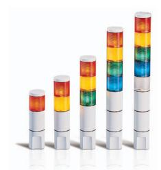
The MicroStat® is a compact, Type 4X status indicator, Type 1 with optional sounder. Ideal for OEM applications, the MicroStat comes pre-assembled as 1-, 2-, 3-, 4-, or 5-high light units. The user selects combinations from five colors: Amber, Blue, Clear, Green and Red. O-rings between each segment provide a water-tight and dust-tight seal. The base of each light can be surface or pipe mounted (3/4-inch NPT).
