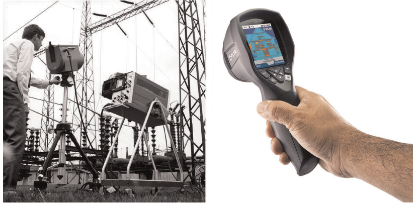
Figure 25.2 LEFT: Thermovision Model 661 from 1969. The camera weighed approximately 25 kg (55 lb.), the oscilloscope 20 kg (44 lb.), and the tripod 15 kg (33 lb.). The operator also needed a 220 VAC generator set, and a 10 L (2.6 US gallon) jar with liquid nitrogen. To the left of the oscilloscope the Polaroid attachment (6 kg/13 lb.) can be seen. RIGHT: FLIR i7 from 2012. Weight: 0.34 kg (0.75 lb.), including the battery.
