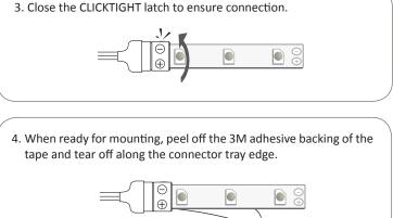
\*All CLICKTIGHT accessories have a Class 2 amperage limit: 60W/5A @ 12VDC; 96W/4A @ 24VDC. CLICKTIGHT connectors are not compatible with wet location tape light. See 'Troubleshooting' for tape light connector issues.
