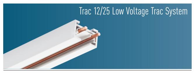
Trac 12/25 combines the 25-amp capacity of 10 gauge conductors with a miniature rigid profile that can be surface mounted or pendant suspended. The system operates off of remotely located 12 or 24-volt transformers. A maximum of 300 watts (12 volts) or 600 watts (24 volts) can be placed per circuit of trac.
