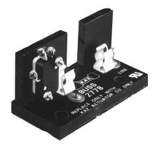
13/32" x 2" (10.3mm x 50.8mm) FUSEBLOCKS WITH MINIATURE SIGNALING SWITCHES 600 VOLT RATING U.L. RECOGNIZED
