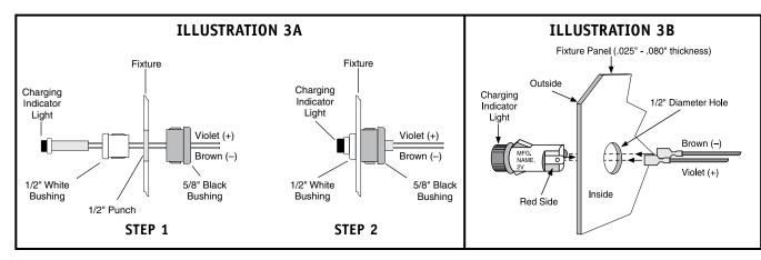
NOTE: After installing the charging indicator light and test switch, mark each with the appropriate label. If a detached charging indicator light is used, connect by matching wire colors and install as shown above.
