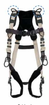
Retrieval An attachment point located on each shoulder strap is used in retrieval operations such as a confined space.
